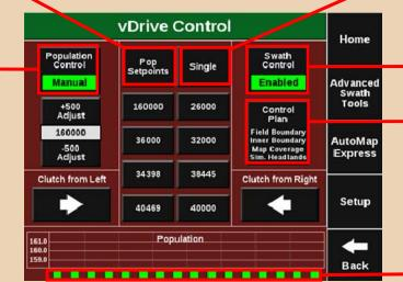
**Swath Control:** This control can toggle between "Enabled" and "Manual." Pressing this button will enable and disable swath control or turn swath off.
